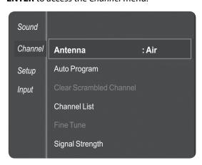
3 Press ▲ or ▼ to highlight **Signal Strength**, then press **ENTER**. The *Signal Strength* screen opens.
